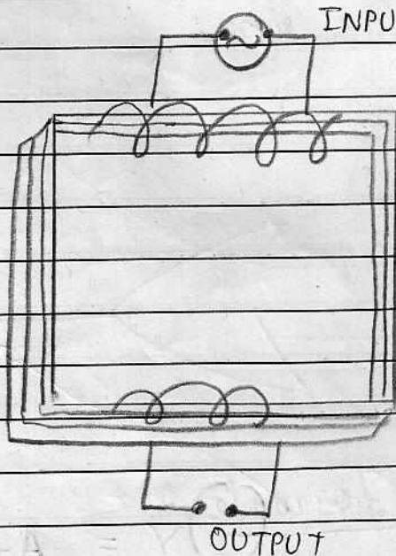
Fig : Step down transformer
