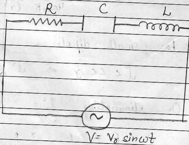
Fig : L.C.R. series circuit
